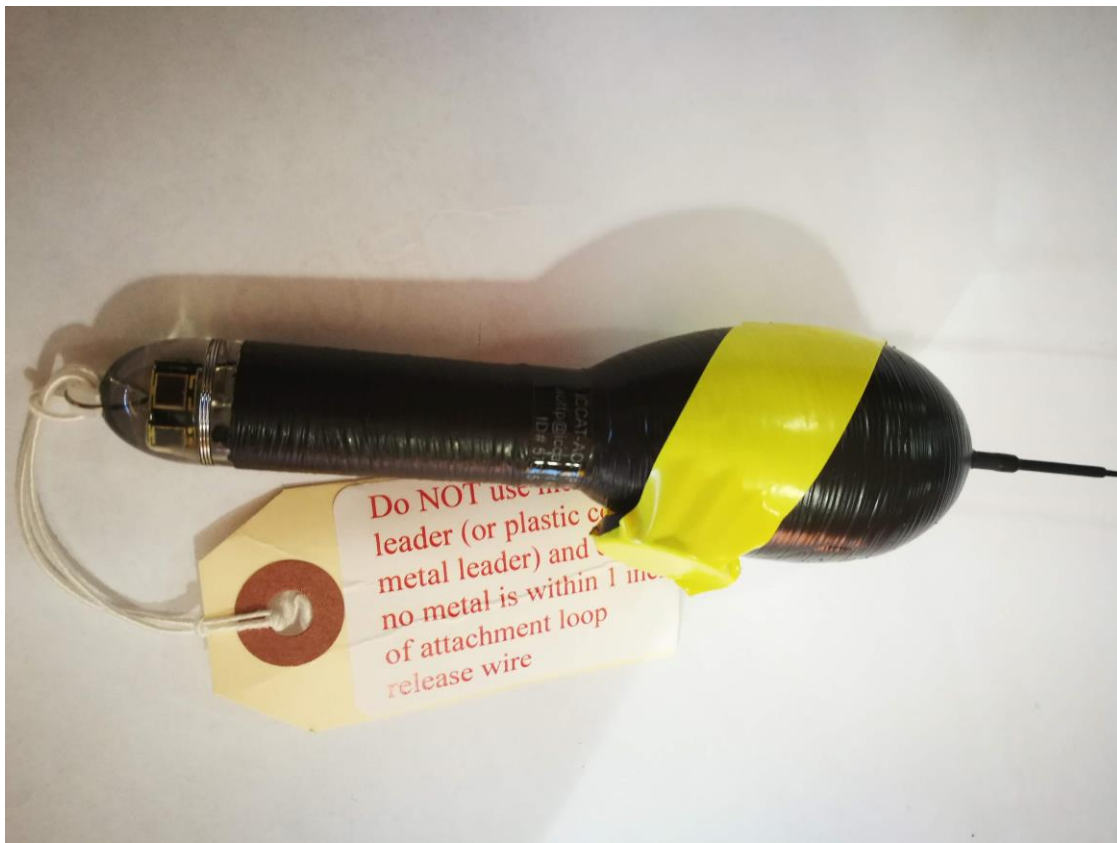
Figure 4: Microwave Telemetry pop-up satellite tag
