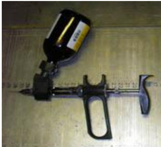
FIGURE 7. INJECTION GUN FOR CHEMICAL TAGGING. NOTE VIAL OF OXYTETRACYCLINE.
