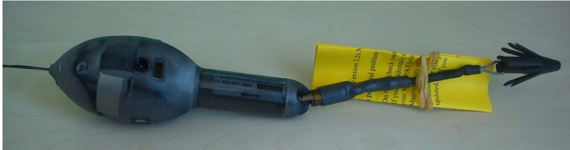
FIGURE 6 POPUP TYPE ELECTRONIC TAG WITH LARGE PLASTIC ANCHOR
