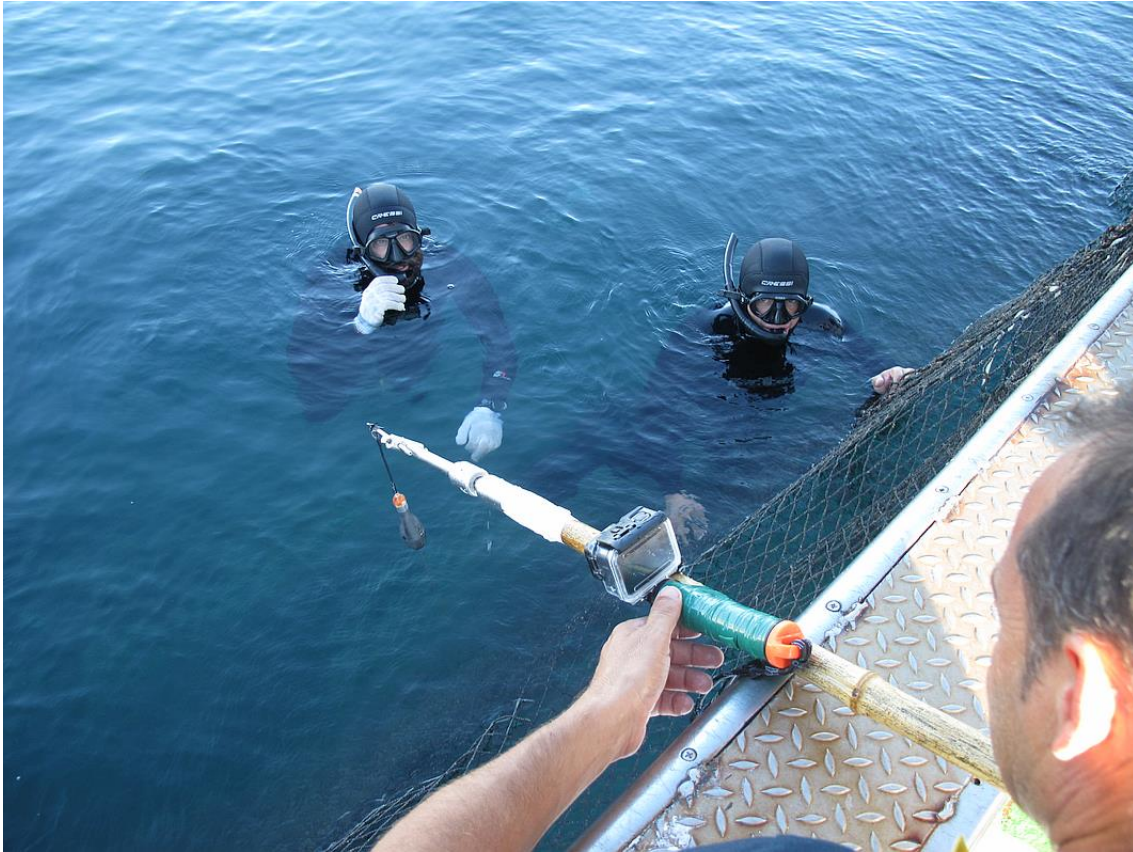
Fig. 4. The tagging coordinator, Mr. Alfredo Poço, handling to a diver the underwater tagging pole with a satellite tag ready to be deployed. A GoPro camera is attached to the pole.
