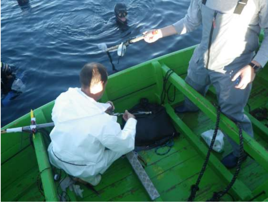
Fig. 4. The tagging coordinator, Mr. Alfredo Poço, preparing a satellite tag in one of the underwater tagging poles. The 2 nd pole is returned for reloading.
