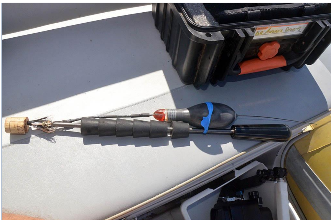
Figure 6 - MiniPAT electronic tag and applicator
