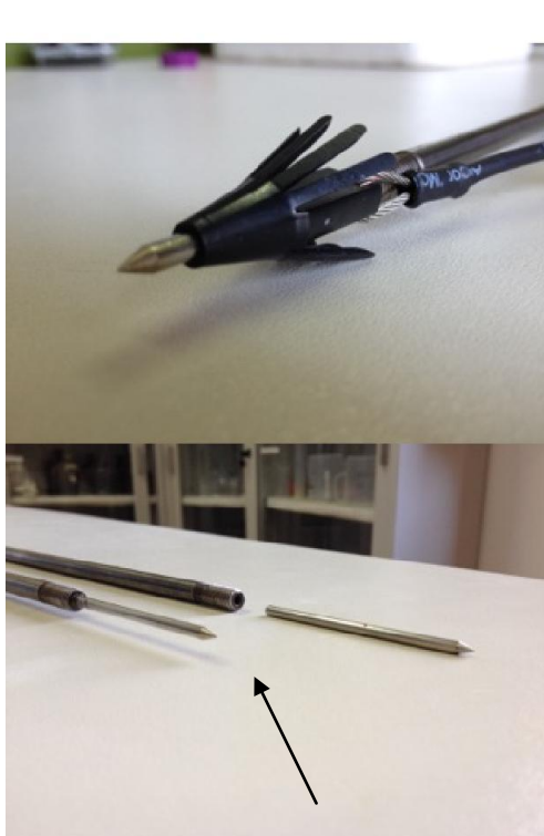
Fig. 5 – Details of the applicator for electronic tagging (shaft was drilled \varnothing 3 mm).
