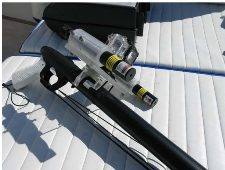
Fig. 10 - Coupled laser used on the speargun for scaling length of bluefin tuna
