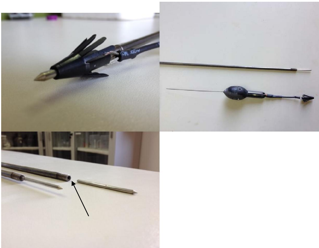
Fig. 4 – Details of the applicator for electronic tagging (shaft was drilled \varnothing 3 mm)
