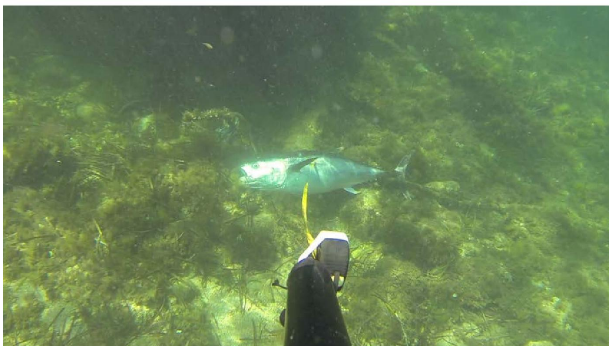
Fig. 15 - Frames showing the trial for validation of length in a 30 kg bluefin at 1 m distance (above) and 2.5 m (below)
