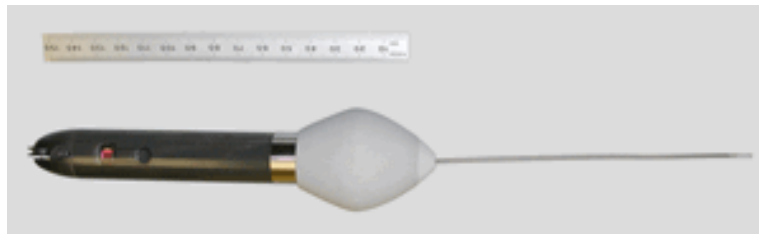
Fig. 3.3.1.2. Mk10-PAT tag (source: Wildlife Computers web site)
