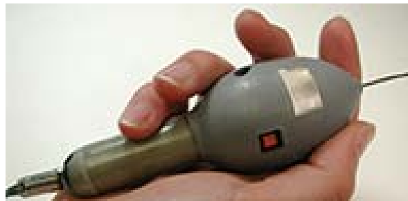
Fig. 3.3.1.3. MiniPAT tag (source: Wildlife Computers web site)
