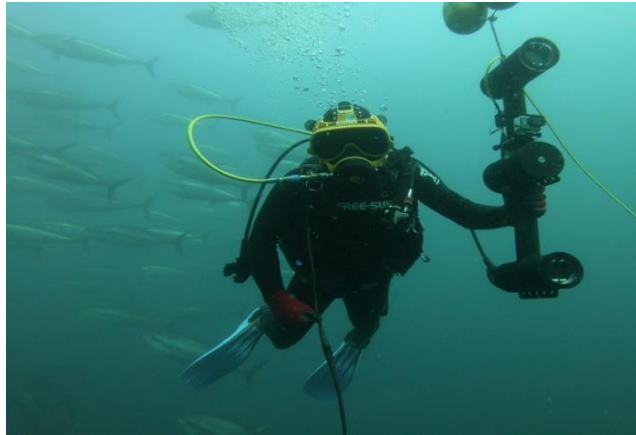
Taking of underwater video by stereoscopic camera
