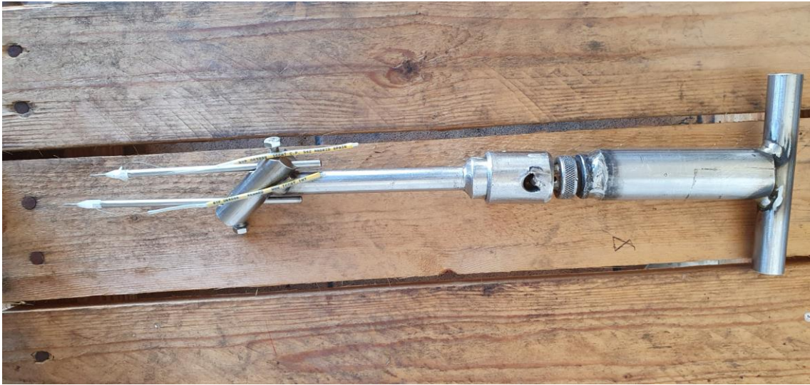
Figure 1 - Tag applicator handle modified for the double tagging used in 2020
