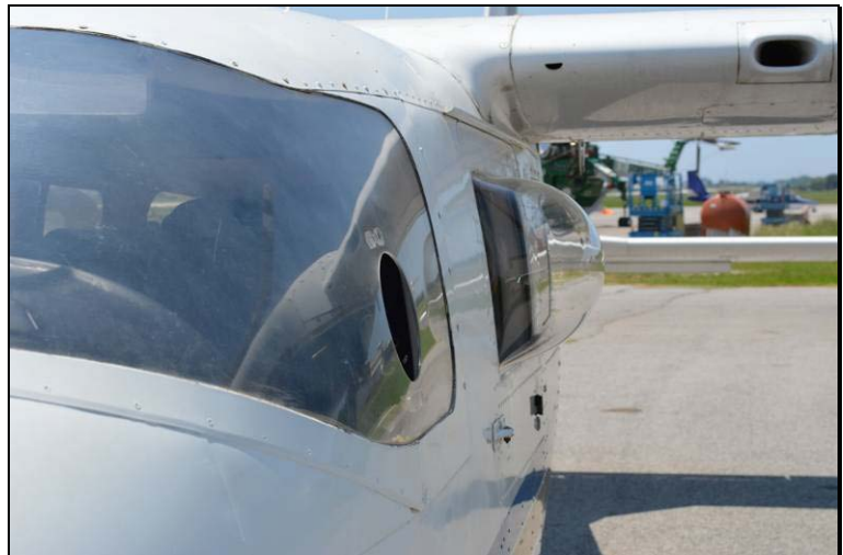
Figure 4 - The I-AGSD aircraft, the bubble windows
