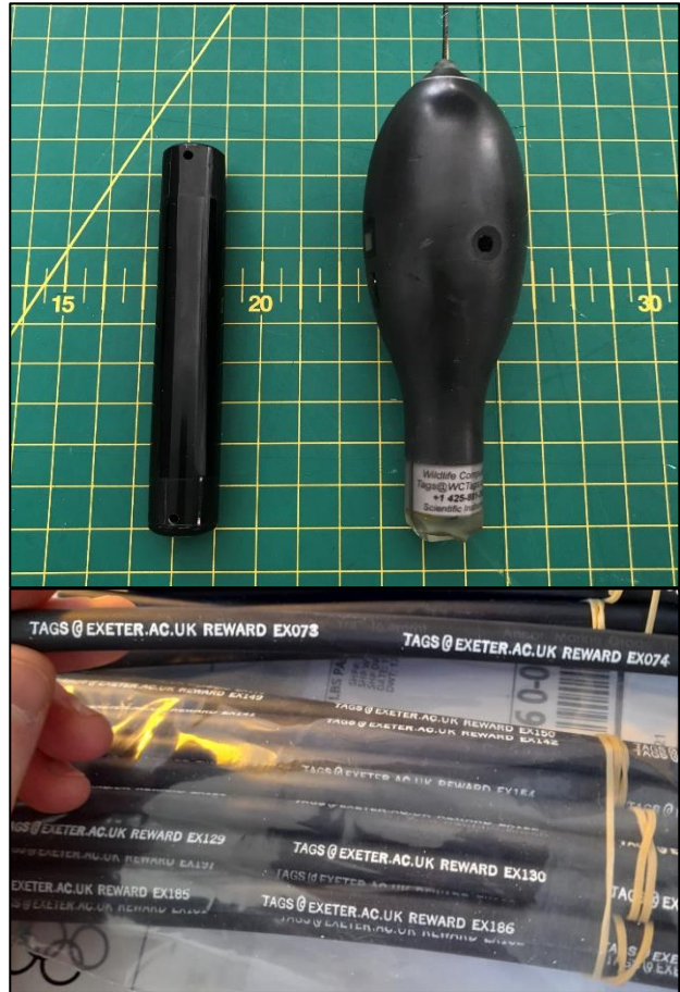
Figure 3. Example of tags deployed in Thunnus UK field operations in 2022 (Thelma HP16 and Wildlife Computers MiniPAT; top panel) and an example of labelled heat shrink used to ID tag tethers (bottom panel; Table 1).
