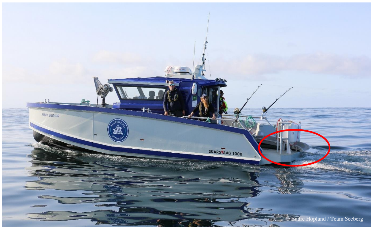
Figure 3: The research vessel “Emmy Egidius” which was used in this study to catch and tag the BFTs. The red circle indicates the movable aluminum landing ramp which was used to pull the BFT on board for tagging. During fishing, the ramp was lifted on board, and it was lowered into the water during tagging.
