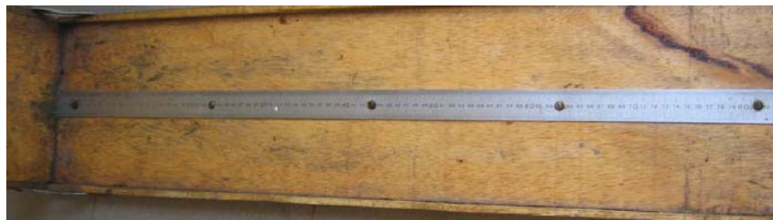
Figure 4.3.2. An example of a measuring board. Picture from Sarralde et al. (2005), reproduced with permission.
