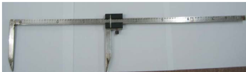
Figure 4.3.1. An example of callipers. Picture from Sarralde et al. (2005), reproduced with permission.
