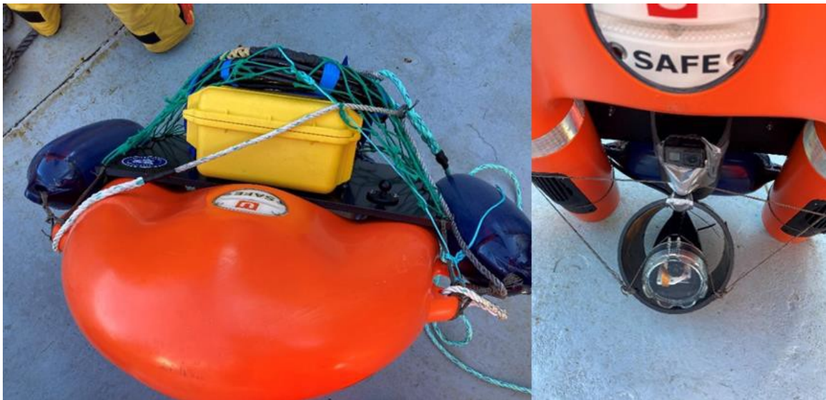
Fig. 6: “USafe” buoy and camera system for monitoring tuna in a purse sein in real-time. Left – the Wireless Mesh Network router inside a water-proof yellow housing, with aerial cable, mounted on type of the “USafe” motorised buoy; Right: the RaspberryPie camera, inside a waterproof housing, mounted beneath the buoy, with a GoPro Hero 7 mounted above. [Image source: Jostein Saltskår].
