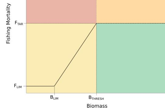
$$F_{mort} = \begin{cases} F_{tar}, \text{if } B_{y-2} \geq B_{thresh} \\ F_{tar} \left( -0.367 + 1.167 \frac{B_{y-2}}{B_{thresh}} \right), \text{if } B_{thresh} > B_{y-2} > B_{lim} \\ F_{min}, \text{otherwise} \end{cases}$$
