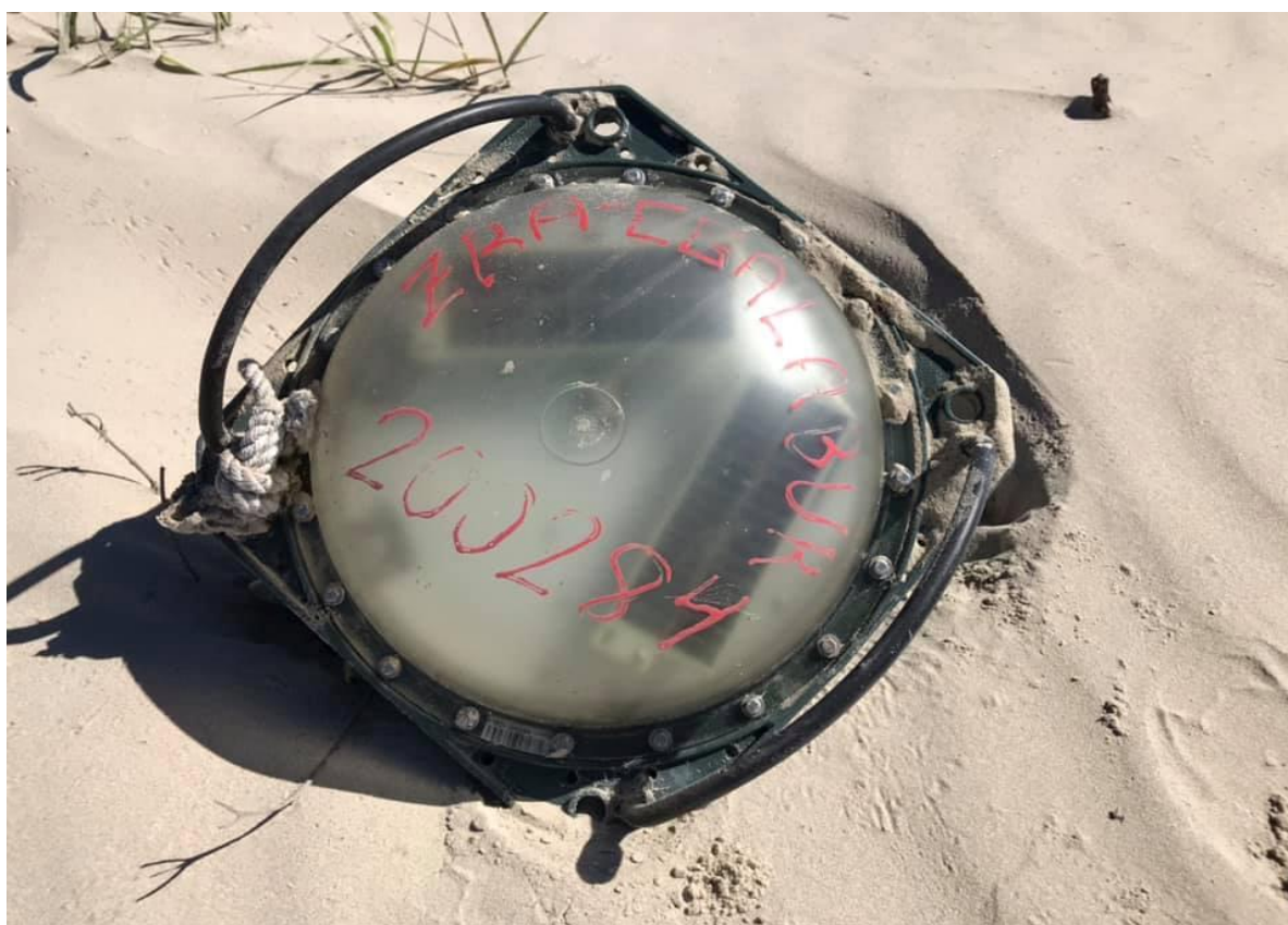
Figure 1. A Marine Instruments M3i model echosounder satellite-linked buoy; an example of a “lone buoy” reported without a FAD raft present. Reported 25 April 2019 from San Jose Island, Texas, United States of America. Photo courtesy of Jace Tunnell.
