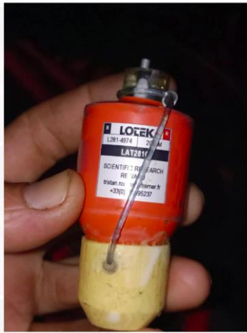
Figure 1. Electronic tag used for long-term deployments. The orange buoy and the white custom-made buoy ensure that the tag can float with all the rigging still attached.
