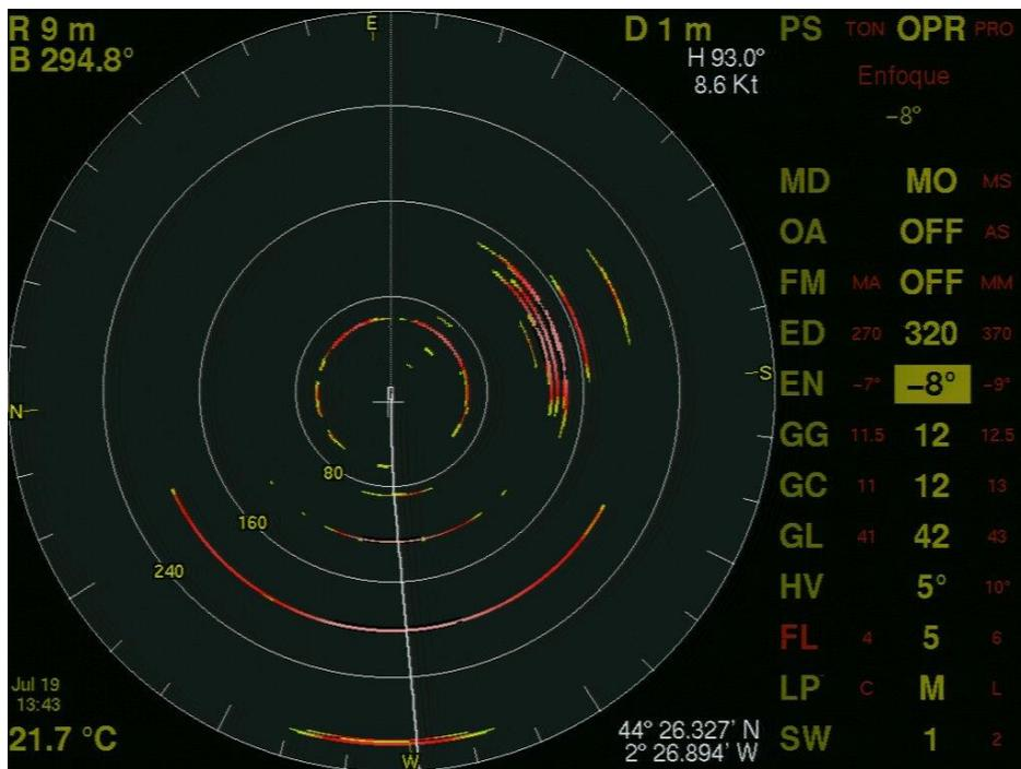
Figure 4. Example of detection of a bluefin tuna school by MAQ sonar (right part of the screenshot).
