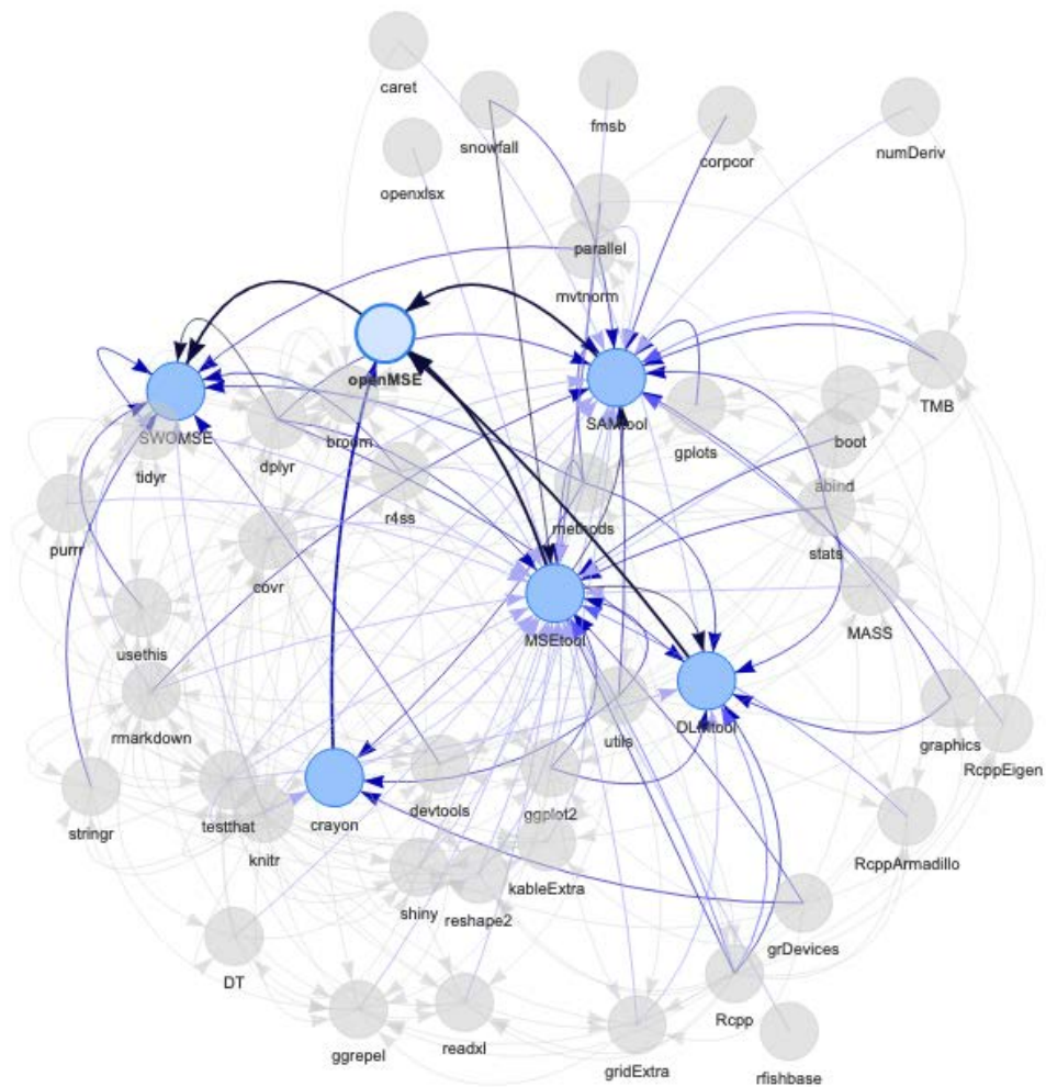
Figure A2. Package dependency directed graph for the openMSE package (indicated by the thicker border on blue circle). This is the same graph as in Figure 1, but with the openMSE package as the focus. Arrow direction indicates contribution (i.e., an arrow from openMSE to SWOMSE indicates that SWOMSE depends on openMSE). [SAM – read package manual for description of the legend here]
