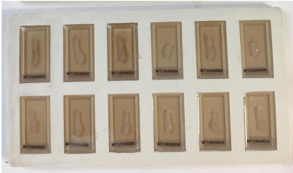
**Figure 6.** Photograph illustrating the mold used to embed otoliths.
