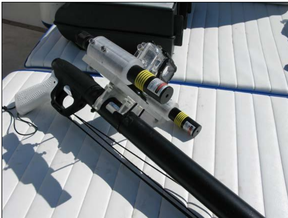
Figure 2. Laser system adopted for size estimate.
