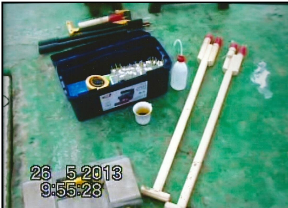
Figure 4. Wooden handles (50 cm length) with two applicators used for double conventional tagging.
