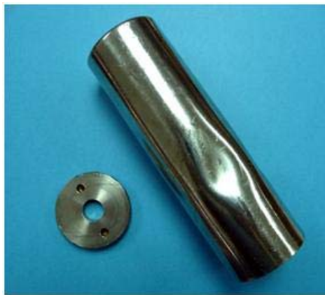
Figure 2b. Protective casing of a sensor (damage during a set).
