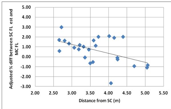
**Figure 11.** Adjusted percentage difference between stereocamera (SC) estimates of the fork length (FL) and measuring calliper (MC) fork length of the fish as a function of distance from the stereocamera.
