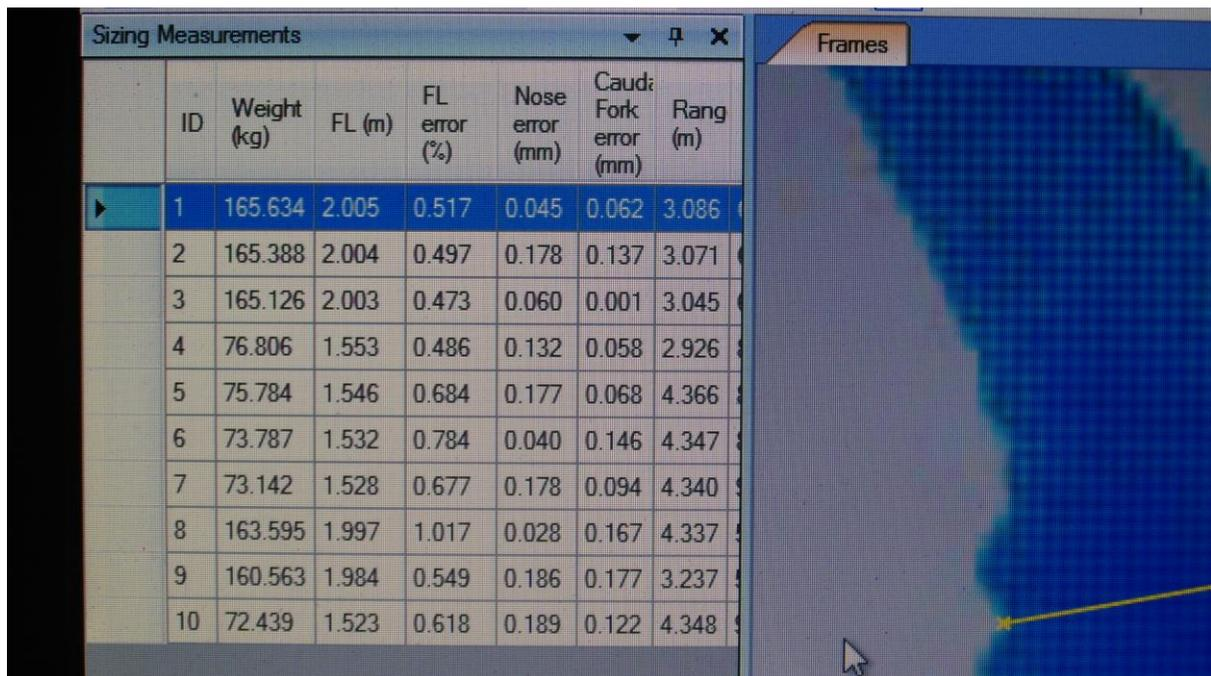
**Figure 4.** Screen shot of AQ1 stereocamera Analyser software showing sizing information obtained with each measurement, including fork length (FL) error, nose error, caudal fork error and range (i.e. distance from stereocamera).
