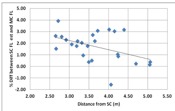
**Figure 9.** Percentage difference between stereocamera (SC) estimates of the fork length (FL) and measuring calliper (MC) fork length of the fish as a function of distance from the stereocamera.
