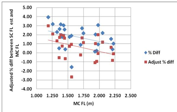
**Figure 10.** Unadjusted and adjusted percentage differences between stereocamera (SC) estimates of the fork length (FL) of the 25 fish plotted against the measuring calliper (MC) fork length.
