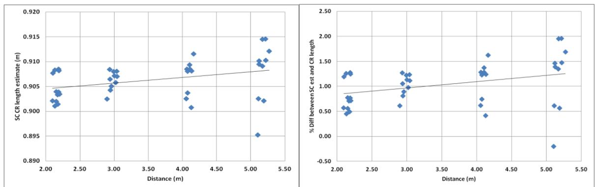
**Figure 5.** Stereocamera (SC) estimates of the length of the calibration rod (CR) plotted against distance from the stereocamera. Data presented as (a) absolute estimate and (b) as a percentage difference between the stereocamera estimate and the actual length of the calibration rod
