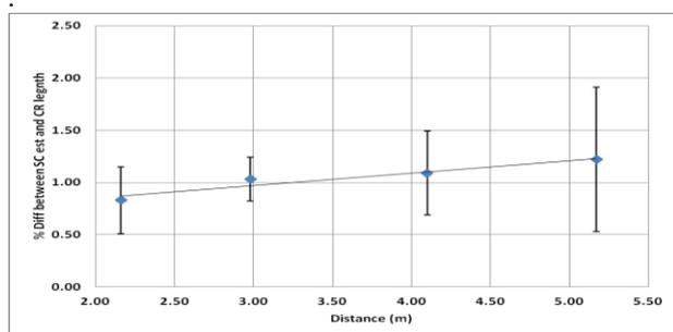
**Figure 6.** Relationship between the average percentage differences between stereocamera (SC) estimated length and calibration rod (CR) length and average distance from the stereocamera. Bars indicate  $\pm 1$  SD.
