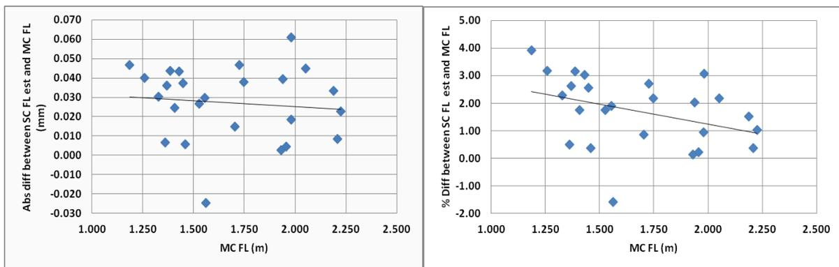
**Figure 8.** Difference between the average stereocamera (SC) estimates of the fork length (FL) of the 25 fish plotted against measuring callipers (MC) fork length. Data presented as (a) absolute difference and (b) as a percentage difference between the stereocamera estimate and the measuring calliper fork length of the individual fish.
