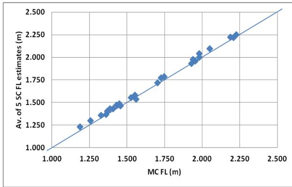
**Figure 7.** Averages of the five stereocamera fork length (SC FL) estimated measurements against the corresponding measuring calliper (MC) fork length of the 25 fish analysed according to the measurement procedure established in Section 3.1.
